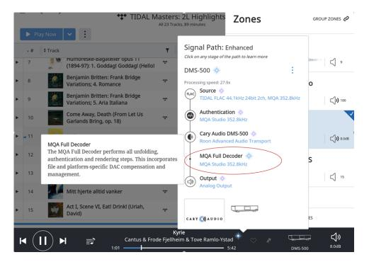
When the DMS-500/550/600 are set as a renderer, you can see from the signal path there are now two-steps to the MQA decoding process. First the Roon Core software will decode the first unfold, then the DMS will render the second and third unfolding. For most circumstances, this is not necessary, and it would be better to let the DMS-500/550/600 decode the full MQA signal.
