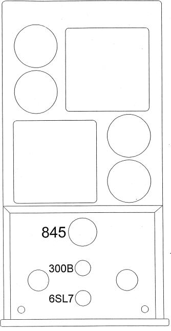
Large pins on 300B tube MUST be inserted into the large holes in the sockets! These pins are on the right side of the amplifier.
