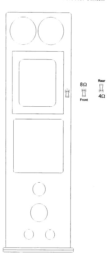
Triode / Ultra-Linear switch settings. Switch is located on the top of the chassis
