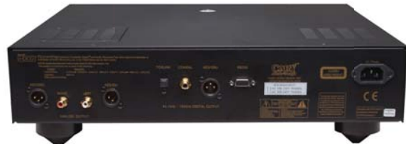
The rear view highlights the adjustable cone metal feet, top panel bubble balance window, the layout of the RCA and XLR analog outputs and the XLR, RCA, and TOSLINK digital output connections.
