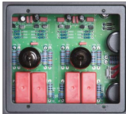
The top view of the 12AU7 output tubes.
